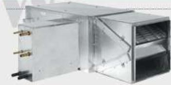
Housed in a heavy-gauge, galvanized steel cabinet, the Horizontal Basic Belt Drive air handler (AH-B) includes coil, forward-curved, dynamically balanced blowers, motor and drive package. Controls and motors are factory-mounted and provided in a single-point power supply. Access doors are provided on both sides of the unit for easy maintenance.
