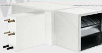
Ideal for applications where a finished cabinet is required, the Horizontal Deluxe Belt Drive (AH-D) is the same unit as our Horizontal Basic model, only finished with a baked-on tough, soft white powder-coat epoxy and subjected to 500-hour salt spray test in accordance with ASTM B117. Access doors are provided on both sides of the unit for easy maintenance. **Also available as Double-Wall (Solid or Perforated).**
