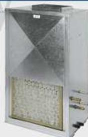
The Vertical Front Return (CV-F) is a high static, ducted vertical fan coil for installation in a closet-type enclosure. The front panel is removable for easy service access to the slide-out blower assembly, with quick-connect plug. CV-F with return-air grille option allows unit to be furred-in. Grille mounts to drywall for easy access without the expense of a closet door. Vertical Front Return Deluxe CV-R also available.
