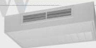
The Horizontal Deluxe (HL-D) fan coil is designed for horizontal exposed ceiling-mounted applications. The HL-D is our basic unit housed in a fully-cased cabinet intended for free-blow exposed ceiling mounting. This unit is ideal for remodel situations where adding AC ductwork is limited. Deluxe cabinets are constructed of cold-rolled steel and finished with a 385 $^{\circ}$  baked-on tough, soft white epoxy powder-coated finish.
