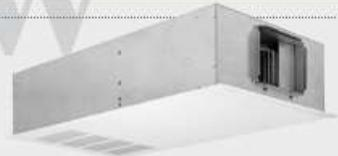
The Cased Flush Horizontal (CH-F) is a horizontally ducted fan coil that aligns flush with the ceiling. Ideal for horizontal applications in apartments, condominiums and motels requiring either a drop-ceiling or soffit installation, the CH-F has a swing-down access panel for fast and easy filter removal and routine maintenance. Bottom return-air is standard.
