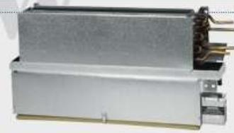
The slim, compact design of our Vertical Basic (LV-B) fan coil is intended for furred-in applications with a field-fabricated, custom enclosure. Housed in a heavy-gauge galvanized steel cabinet, insulated with 1/2" thick neoprene coated fiberglass, this reliable fan coil is ideal where most any through-the-wall installation is desired.
