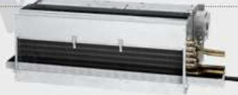
Designed for furred-in, under-the-window applications, the Low Silhouette Vertical Basic (LS-B) stands only 15 1/2" high and accommodates a field-furnished and installed decorative enclosure that conceals the unit. The basic unit consists of a chassis, fan deck, drain pan, throwaway filter and a top-discharge duct collar.
