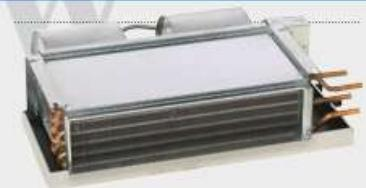
The low profile and flexible design of the Horizontal Basic (LH-B) fan coil is ideal for multiple applications. The slim, compact design is well suited for drop-ceiling, closet, hallway and other concealed applications. The LH-B comes with a powder-coated epoxy drain pan and a wide range of coil, motor and controls options. These models have no exterior cabinet.
