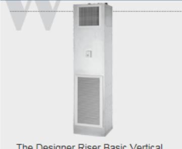
The Designer Riser Basic Vertical Stack (DR-B) is for concealed applications along walls and in corners. This model comes standard in an extended 97 galvanized steel cabinet, insulated with 1/2" thick neoprene-coated fiberglass. Like the ER-B, this unit features a 1/2" OD copper tube coil, slide-out blower assembly with quick-disconnect plug, insulated drain pan and filter.
