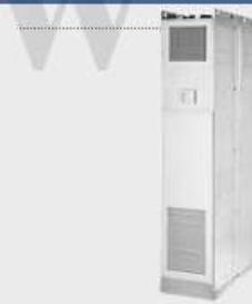
The TwinPack is a master/slave combination that is pre-piped and housed in a common cabinet assembly at the factory. TwinPack Vertical Stack units include a UL 1-Hour Through Penetration Firestop W-L-7089 system. Local codes may dictate exact amount and placement of drywall. Each unit has its own set of valves and controls.
