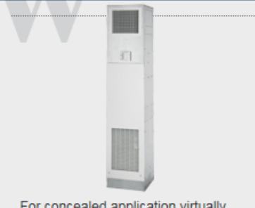
For concealed application virtually anywhere in the room, the Easy Riser Basic Vertical Stack (ER-B) comes standard in a heavy-gauge 88 galvanized steel cabinet, insulated with 1/2" thick, neoprene-coated fiberglass. This standard unit features a 1/2" OD copper tube coil, slide-out blower assembly with quick-disconnect plug, insulated drain pan and filter. Risers are ordered separately due to size changes throughout the building.
