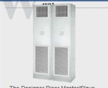
The Designer Riser Master/Slave Vertical Stack units have the same internal components as our Basic model, yet are designed to share a common riser set. The Master/Slave combination features two separate units piped to a common set of risers, each with individual valves and controls. The ER-M and ER-S come in a 97 galvanized steel cabinet.
